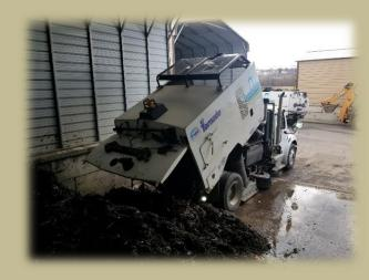
designed to remove fine road dust and pollutants stemming from asphalt, wearing of brake discs/pads or tires, and large discarded items. (Pictured: 79,020 lbs. of debris removal from a 4-day sweep in Wilkes-Barre)
