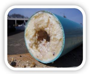
Grease trap FOG refers to fats, oils and grease. When poured down a drain, FOG cools and hardens as it flows down the sewer pipe and attaches to solids normally found in the sewers forming clumps. These clumps eventually stick to the sides of the pipes and slow the flow of sewage.
