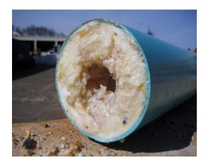
Fats, oil and grease (FOG) hardens as it flows down the sewer pipe and attaches to solids normally found in the sewers forming clumps. These clumps eventually stick to the sides of the pipes and slow the flow of sewage.
